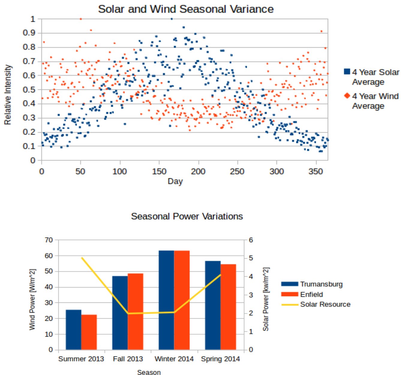
Figure 37 (a) Relative wind intensity vs. relative solar intensity for Harford, NY and (b) Solar power seasonal variations represented by the yellow line compared to wind power seasonal variations represented by the two bar graphs at two locations 29
