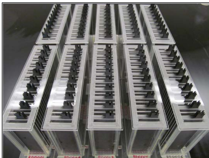
Figure 65. 1-kW Zinc-air Prototype (Photo courtesy of EOS Energy Storage)
