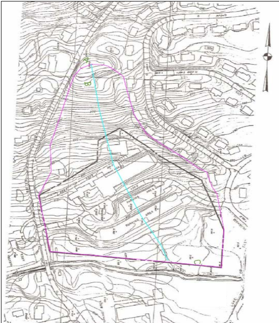
Figure 2: Delineated Watershed and Hydraulic Path - Predevelopment
