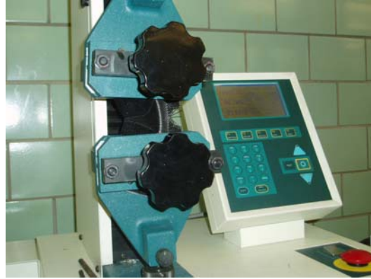
Figure 9-40b Geotextile Testing (Trapezoidal Tear Test)
