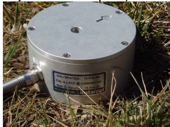
Figure 9-58d Vibration Monitoring (Triaxial Geophone)
