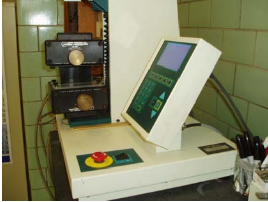
Figure 9-40a Geotextile Testing (Grab Strength Test)
