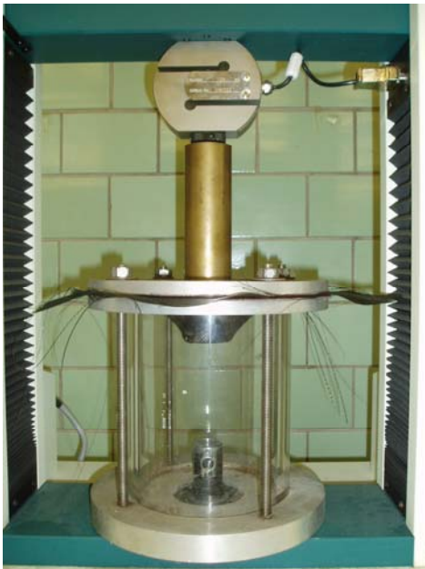
Figure 9-40c Geotextile Testing (50 mm Puncture Test)
