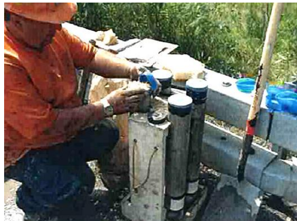
Figure 9-4d Undisturbed Sampling (Capping Sample and Securing for Delivery to Lab)
