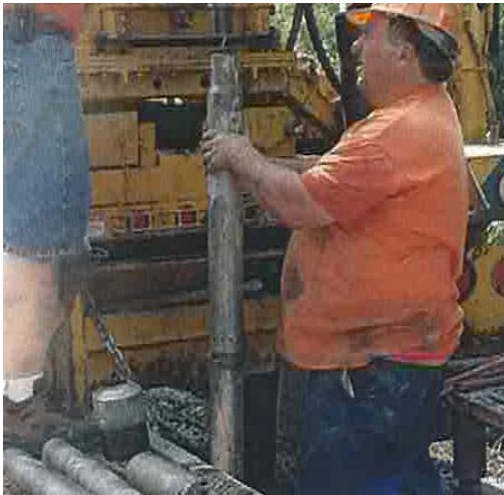
Figure 9-4a Undisturbed Sampling (Setting Sampler)
