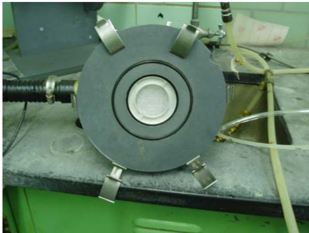
Figure 9-40e Geotextile Testing (Permittivity Test- Geotextile in Ring)
