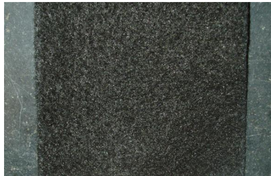
Figure 9-39d Needle Punched NonWoven (SI GeoSolutions GEOTEX 1001)
