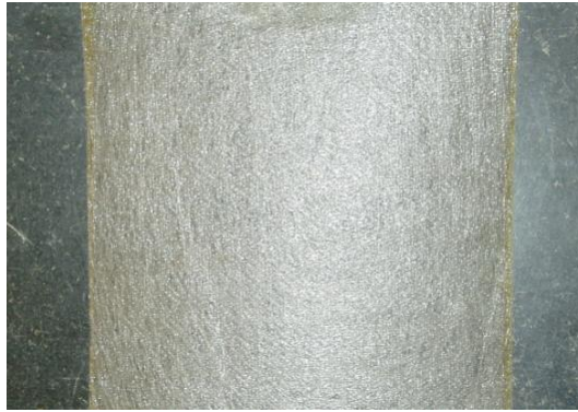
Figure 9-39e Heatbonded NonWoven (BBA FiberWeb Typar 3401G)
