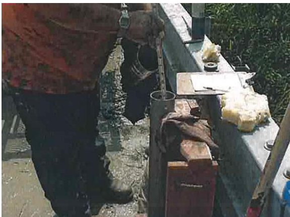
Figure 9-4c Undisturbed Sampling (Sealing Sample with Wax)
