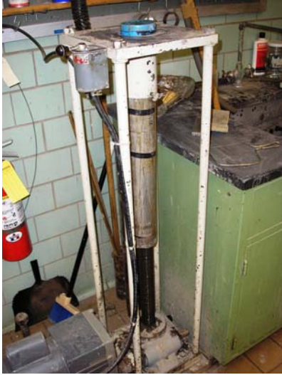
Figure 9-4e Extracting Undisturbed Soil Sample in Lab
