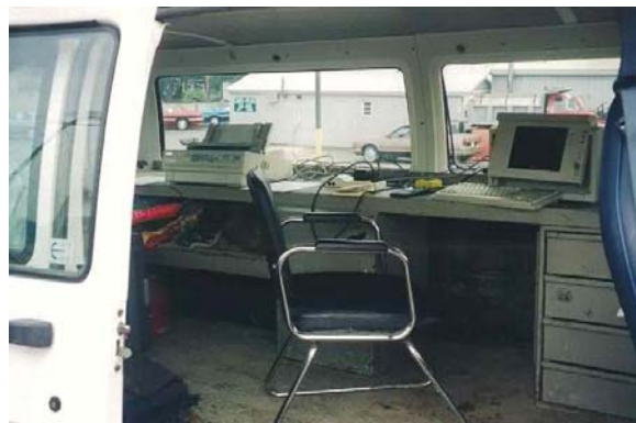
Figure 9-55g Crosshole Sonic Log Testing (Mobile Test Lab)
