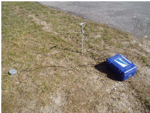
Figure 9-58a Vibration Monitoring Set-Up
