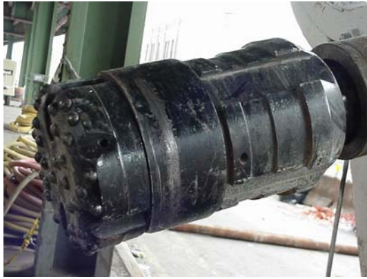
Figure 9-57b Micropile Installation (Down-The-Hole Hammer)
