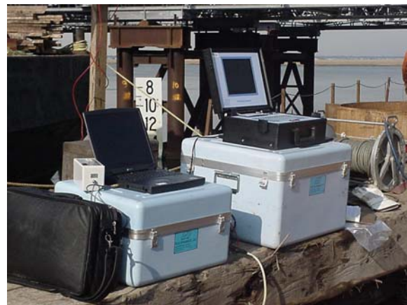
Figure 9-56d DPLT: Pile Driving Analyzer (Pile Dynamics, Inc.)
