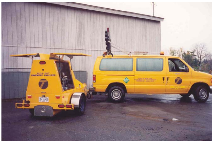
Figure 9-11 Falling-Weight Deflectometer (FWD)
