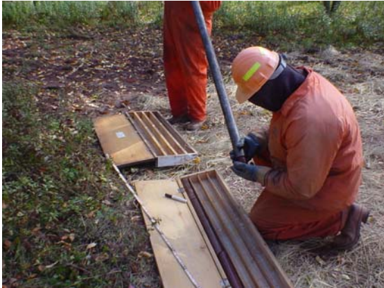
Figure 9-6a Extracting Rock Core Sample
