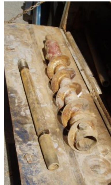
Figure 9-3b Hollow-Flight Auger with Split Spoon Sampler
