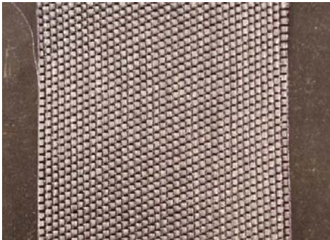
Figure 9-39c Combination Monofilament/ Fibrillated Yarn Woven (WEBTEC Terra Tex HPG 16)
