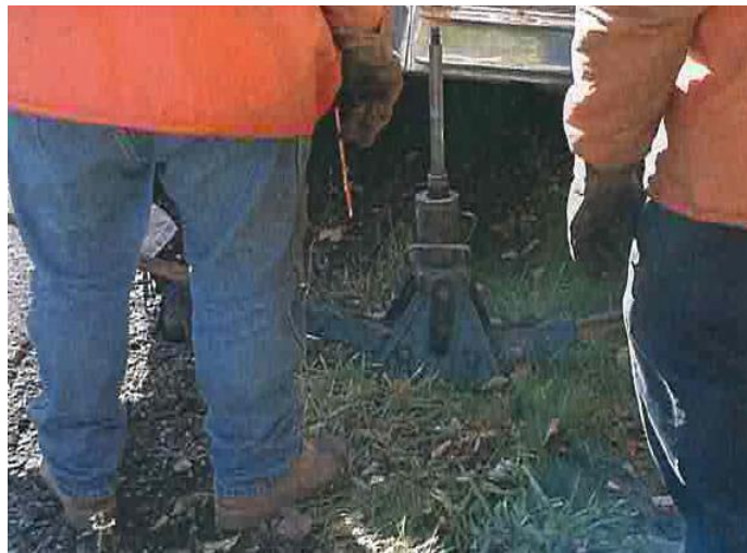
Figure 9-5a Probe Hole (Jack to Extract Rods)
