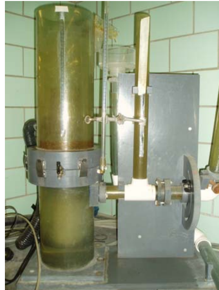
Figure 9-40f Geotextile Testing (Permittivity Test)
