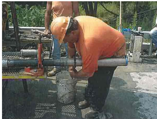
Figure 9-4b Undisturbed Sampling (Breaking Down Sampler)
