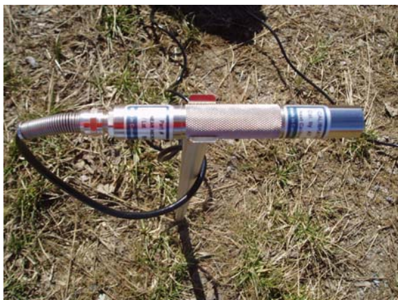
Figure 9-58c Vibration Monitoring (Microphone)
