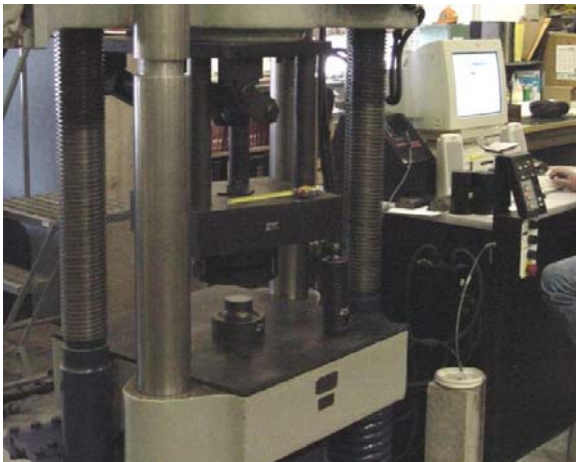
Figure 9-6e Unconfined Compression Test
