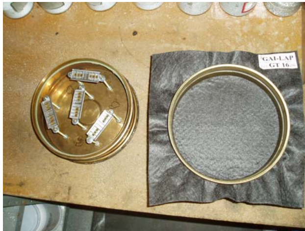
Figure 9-40g Geotextile Testing (Apparent Opening Size Test)
