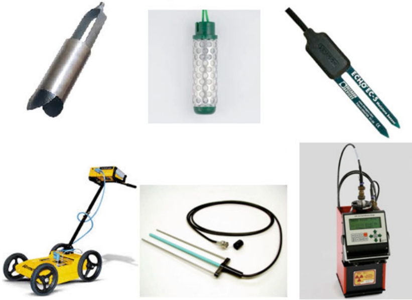
Fig. 6.3 Soil moisture sensors. Top row: Gravimetric [13], resistive (Watermark) [22], and capacitance [18]. Bottom row: GPR [19], TDR [37], and neutron probe [14]
