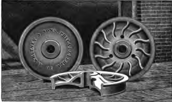
Fig. 51.—Cast-iron Car Wheels.
