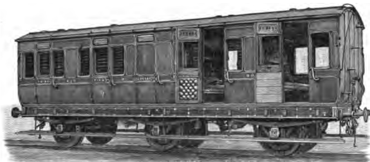
English Railway Carriage, Midland Road. First and Third Class and Luggage Compartments.
