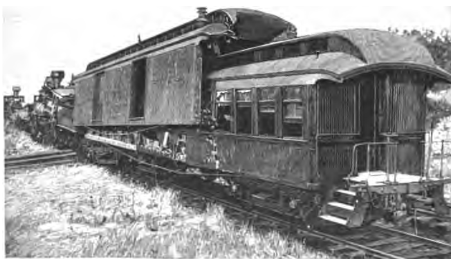
Some Results of a Butting Collision—Baggage and Passenger Cars Telescoped.
