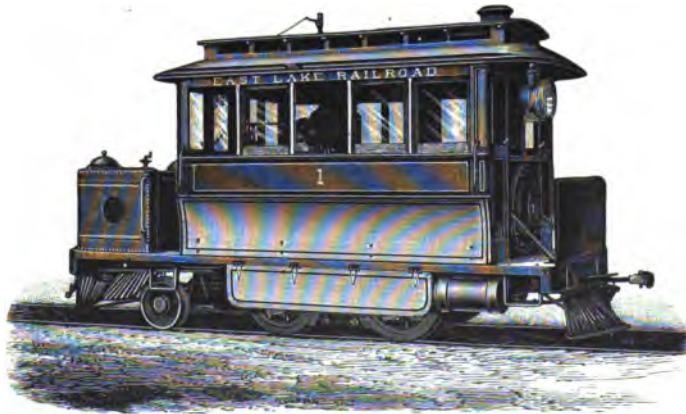
Fig. 13.—Locomotive for Street Railway. By the Baldwin Locomotive Works.
